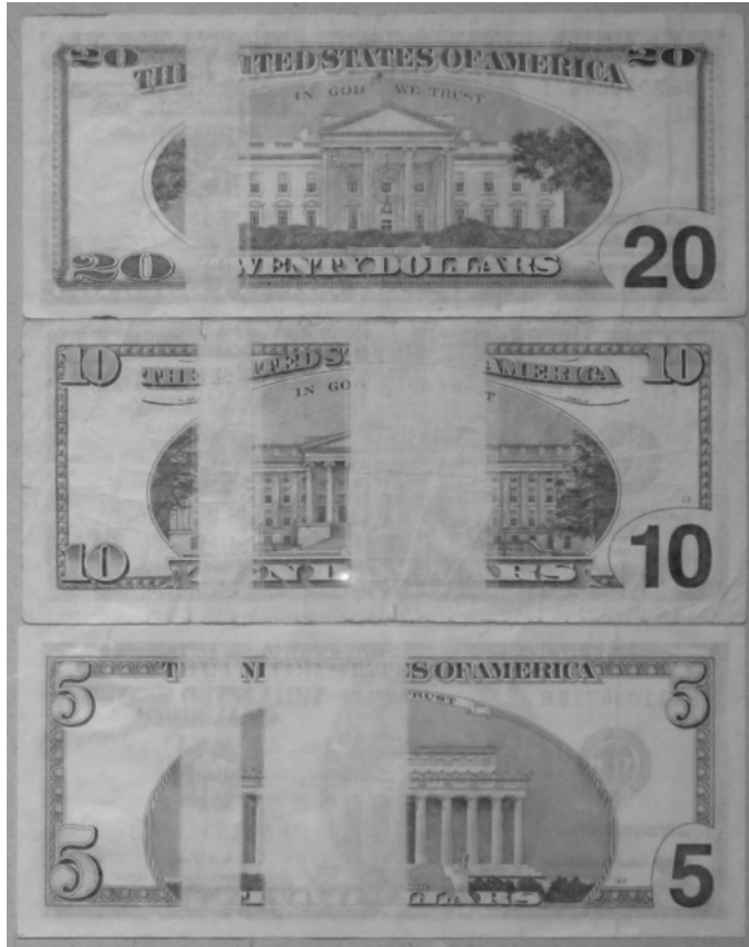
Bills viewed under an infrared camera, revealing the blank bands. There are different band patterns for each denomination.
