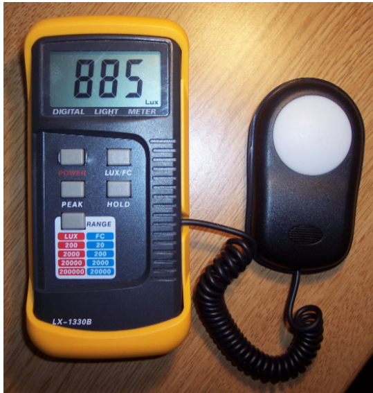
Example of a light meter. The left part gives the reading, while the right part receives the radiated or reflected light.
