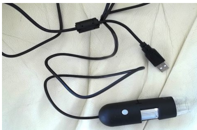
This is an inexpensive digital microscope that plugs into the computer. The image appears on your screen and you can take microscopic photos.
