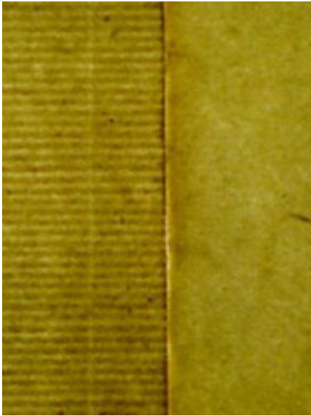
Laid paper (left) and its gridion lines next to wove paper (right)
